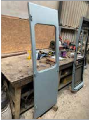
New outer skins fitted.
