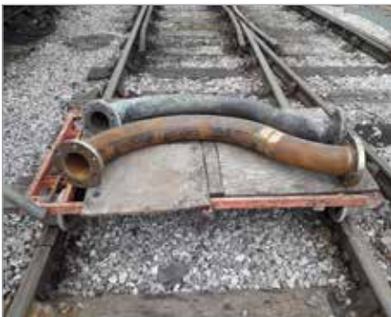
New and Old Steam Pipes
