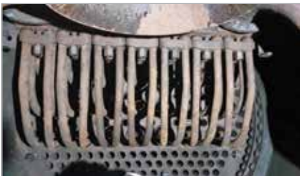
Top: Superheater elements are long! Fitting being done inside the maintenance shed.
